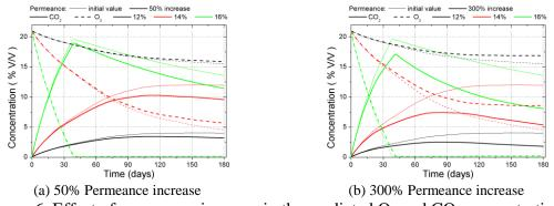
Figure 6. Effect of permeance increase in the predicted O<sub>2</sub> and CO<sub>2</sub> concentrations
