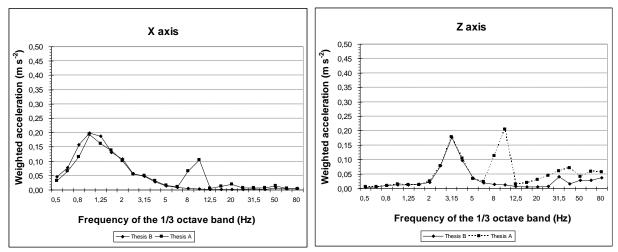
Figure 4. Values of the weighted accelerations found on the tractor's main frame with the oscillating metal plate in action (thesis A) and steady (thesis B).
