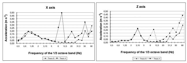
Figure 3. Values of linear accelerations found on the tractor's main frame with the oscillating metal plate in action (thesis A) and steady (thesis B).
