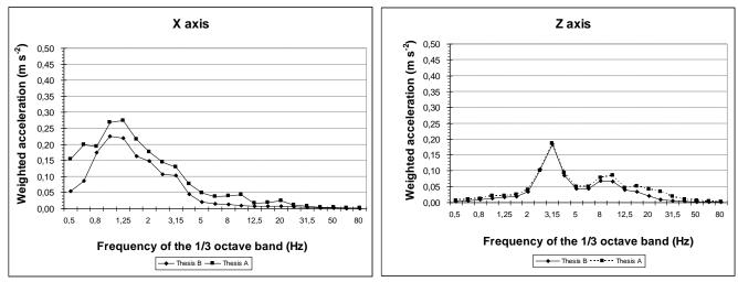
Figure 5. Values of the weighted accelerations found on the driver seat with the oscillating metal plate in action (thesis A) and steady (thesis B).
