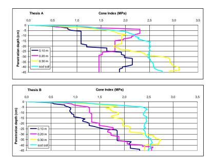
Figure 2. The average C.I., for each theses, in the three positions from the center of the furrow.
