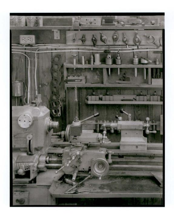
Little John 5" lathe (6" UK standard), c. 1950; Manufactured by Ragland Engineering, Nottingham, UK; Bought in West Sussex, 1960; Rack of lathe chucks, dogs, and collets on the wall behind
