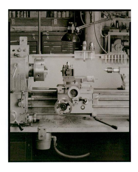
Lux-On Gap-bed lathe (8" over carriage US standard, 13" swing over bed, 20" over gap); Taiwan, 1982; Bought in 1982
