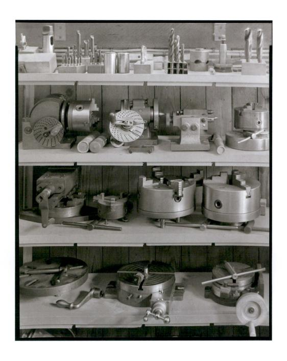
Boring bars, dividing heads, rotary tables, chucks, collett fixtures; Arranged in memory of L'Encyclopedie, Diderot et D'Alembert
