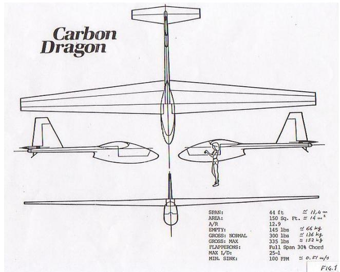
**Figure 1** The Carbon Dragon schematic
