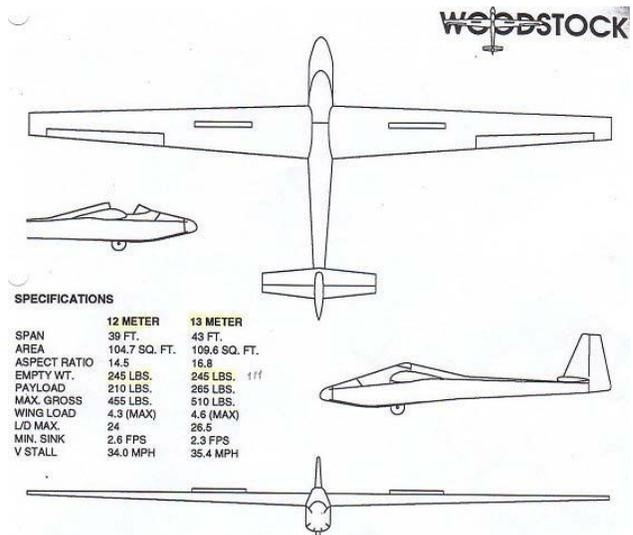
**Figure 5** Schematic of the Woodstock
