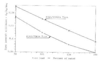
FIGURE 9. Lateral stiffness of two types of tires as a function of load.
