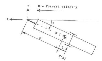
FIGURE 1. Trailer schematic for deriving equations of motion.
