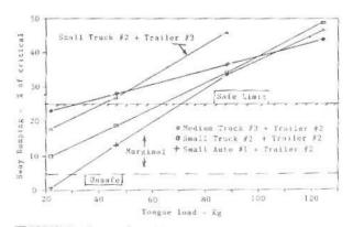
FIGURE 7. Sway damping of trailer #2 towed at 100 km/hr.
