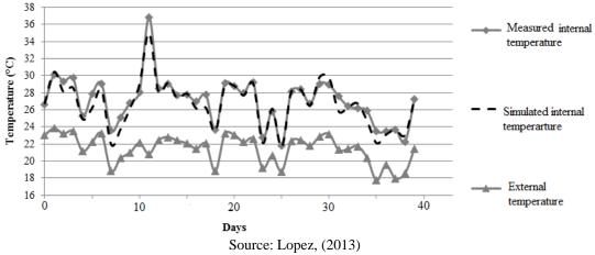
Figure 2. Measured and simulated temperatures for ventilated greenhouse in Cartago
