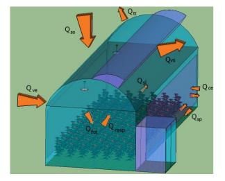
Figure 1. Energy losses and gains in a ventilated greenhouse.
