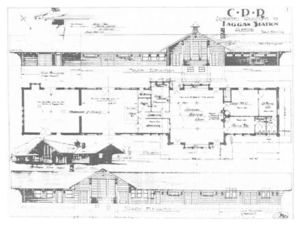
Drawings prepared in 1909 for an addition to the railway station in Laggan, Alberta. The original station was constructed betwen 1885-1887 and moved to Heritage Park, Calgory, in 1976. (CIHB)
